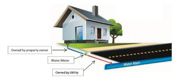
NOTE: Under SB 427 and previous California regulations, the sections of the service line titled *"Owned by Utility"* and the *"Water Meter"* are included in California's definition of a *"service line."* The EPA's new LCRR expands the definition of *"service line"* to also include *"Owned by property owner"* such that the entire line, regardless of ownership, is required to be included in a water system's inventory.
